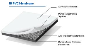
IB Roof Systems PVC roofing materials are designed to protect and extend the life of your building's roof.
