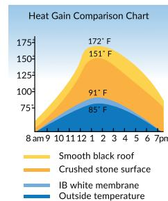
A white IB Roof Systems membrane can reduce your energy consumption and your rising electric bills, by reflecting up to 90% of the heat that normally enters a building through the roof. An IB Roof Systems roof will lower your building's heat gain, and possibly pay for itself.
